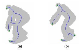
Figure 2. (a) Loop (b) Corner and redundant line
